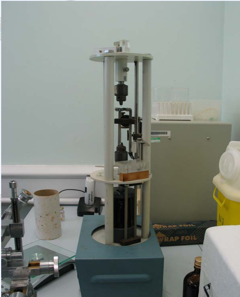
Standard puller is used to pull long pipettes
