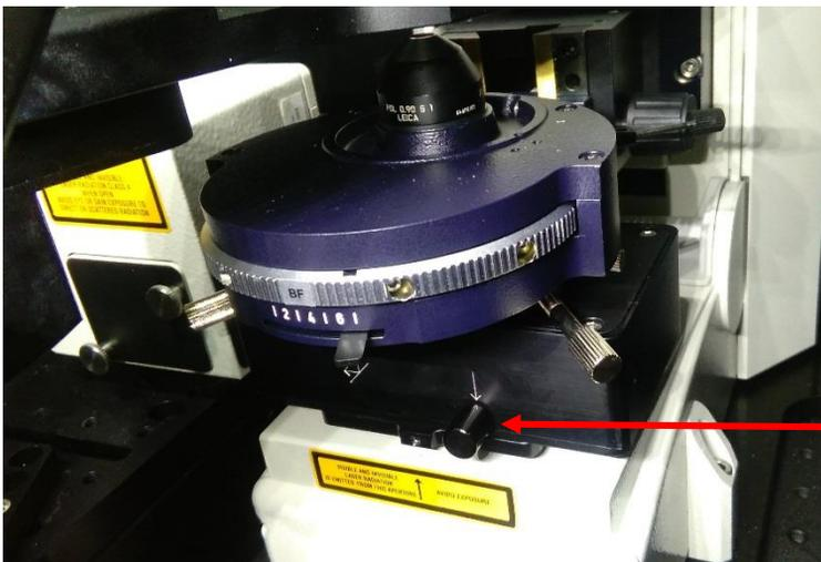
Slider in current position allows you to view brightfield images down the eyepieces.
