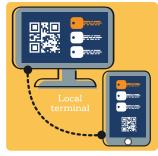
Keys generated locally at node transferred to mobile device via desktop terminal connection.
