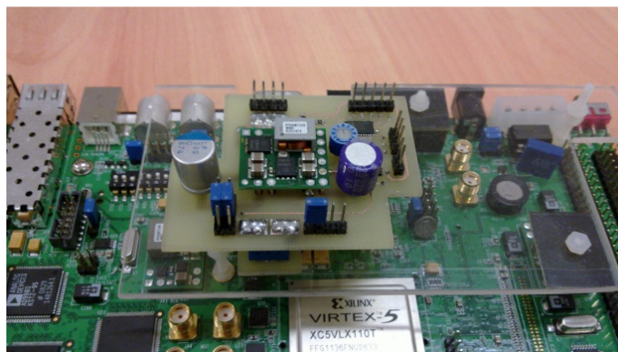
Figure 1. Voltage scaling PCB
