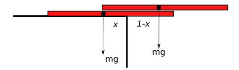
In either case, we find that a balance can only be obtained by setting that the mass times length on the left must equal to mass times length to the right of the pivot point. So, referring to the diagram.
