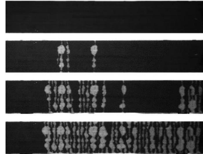
Fibre fragmentation in thin carbon layer of glass/carbon hybrid
