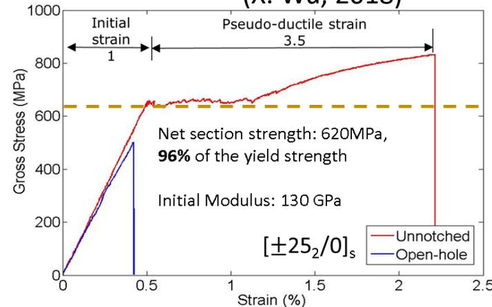
Pseudo-ductile thin ply angle plies + reduced notch sensitivity
