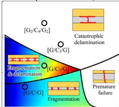
damage mode map for pseudo-ductile design
