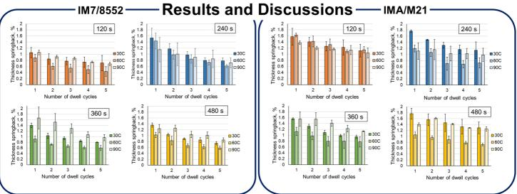
For both material systems, springback decreases with each successive cycle. However, the largest springback was observed at different compaction temperatures for each material system. The compaction temperature also affects the springback in these material systems. This information can be used to update current manufacturing practices, as well as develop numerical models, thus helping to drive improvements in the quality of the final part after manufacture
