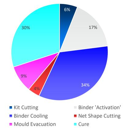
Evaluation of the time cost of each stage of the fabrication of a simple automotive part manufactured utilising HP RTM
