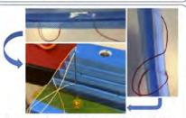
Detachable skin design - Stitching of stringers to the spine using aramid thread. Channels and holes in the stringer are needed to accommodate the
