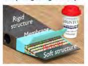
PLA structure in additive manufacturing. Coffee grinds as granular media and silicone membrane
