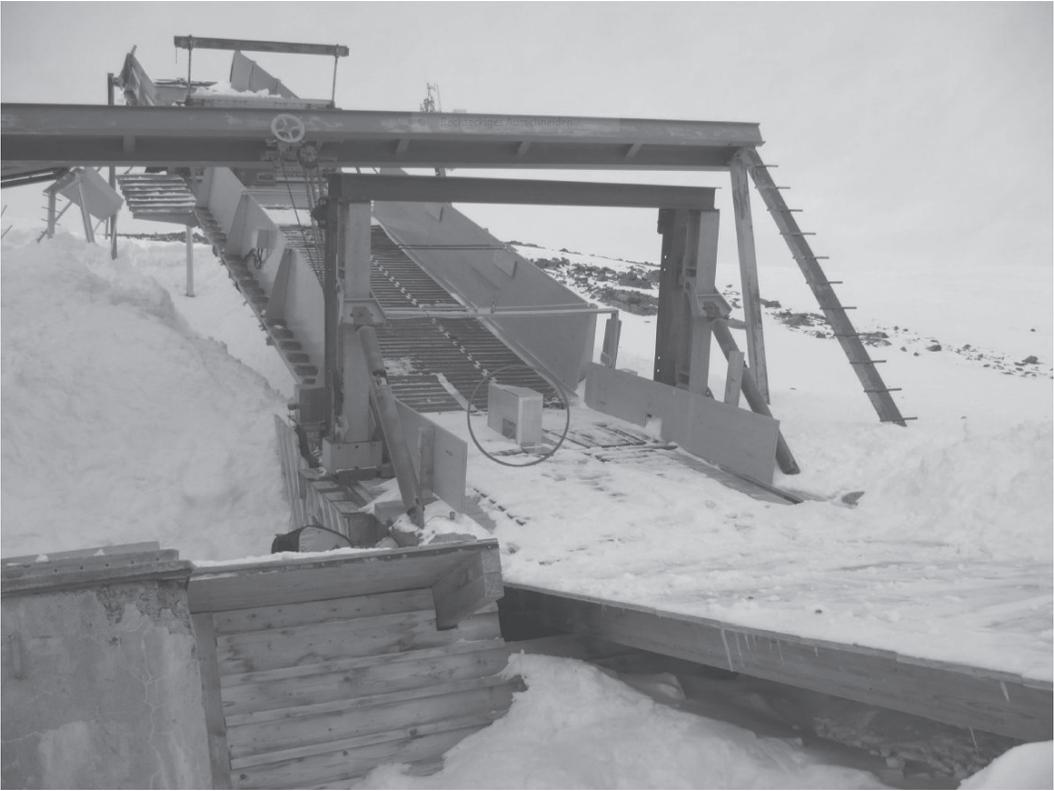
**Fig. 1.** Photograph of the SLF snow chute at Weissfluhjoch, in Davos, Switzerland: the circle in the centre of the picture indicates the half-wedge containing the optical sensor array (photograph, M. Schaefer, SLF)
