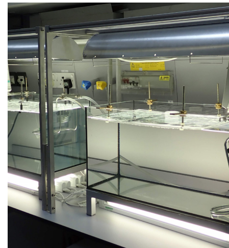
Experimental system for stomatal bioassays Photo credit: Helen Harper
