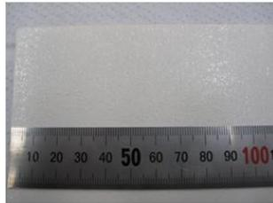
B-stage un-cured epoxy resin film with release paper (30g/m<sup>2</sup>, 25μm)
