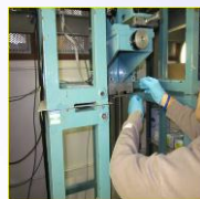
c) The glass rod softened and spun through the orifice.
