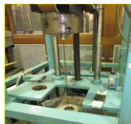
b) Glass rod was gripped by chuck before being drawn.
