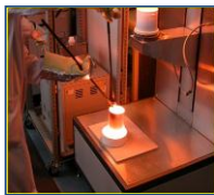
a) Transfer of platinum crucible at 1600°C to drawing furnace at 1240°C
