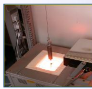
b) MAS fibre was up-drawn as the appropriate melt viscosity
