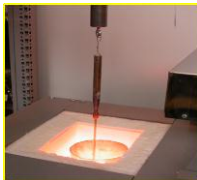
a) Rods up to 1.5m long with 5 mm diameter were produced by dipping a metal rod into molten glass
