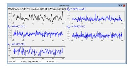
It is easy here to pick out that  $\beta_0$  which is pushed up the hierarchy has been updated using Gibbs sampling whilst  $\beta_1$  is using Metropolis Sampling. If we compare the ESS for all parameters with those from WinBUGS earlier we see the results given in the 3rd and 4th columns below:
