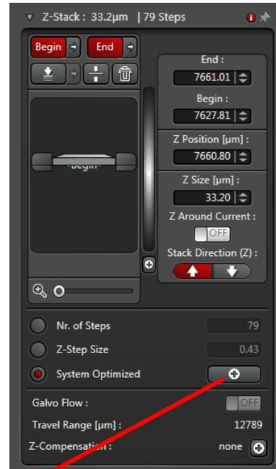
Note that it is not always necessary/desirable to capture at the optimized Z resolution settings (due to the time taken, photo bleaching etc.).
