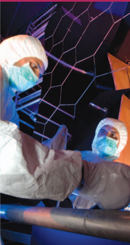
The mirrors of the RICH2 detector of the LHCb experiment are meticulously assembled in a clean room.
