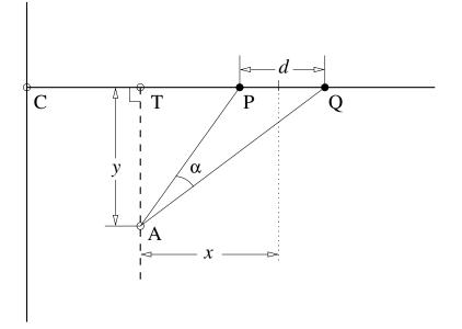
Suppose that the post width d and the distance x of T from the centre line of the pitch are fixed. We want to find the optimum value of y, which maximises  $\alpha$ .
