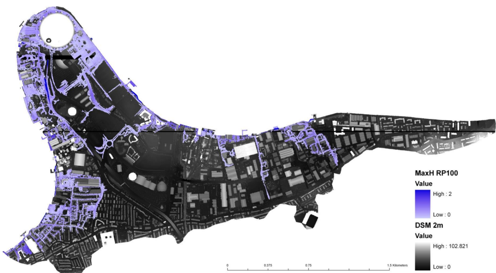
Figure #1: Maximum predicted water depth throughout the simulation for \Delta x = 2 m for the 1-in-100 year return period flood
