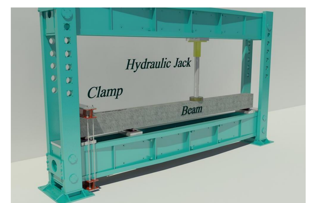
Test on CaFC-Reinforced Continuous Beam
