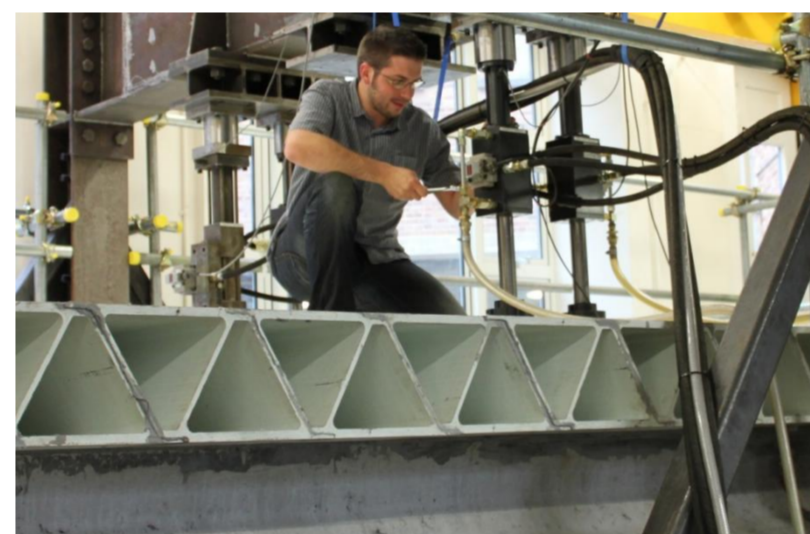
GFC Decking in Specimen
