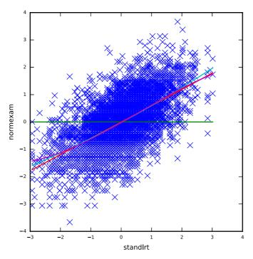
The graph includes best fitting curves for a constant, linear, quadratic and cubic relationship between normexam and standlrt. In this case a quadratic relationship is most appropriate and you might consider including a squared term in the predictor list.
