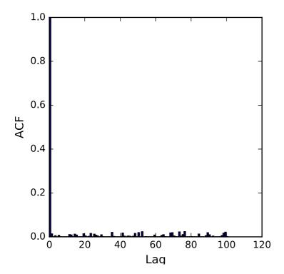
Here the acf value at lag 1 is  $\rho = 0.0132$  and as MCMC algorithms should produce chains resembling an auto-regressive process of order 1 i.e. the value at the current iteration only depends on the last iteration, the value at lag 2 should be approximately  $\rho^2$  (0.000175) and in reality it is -0.00353. Here the chain is only a little correlated.
