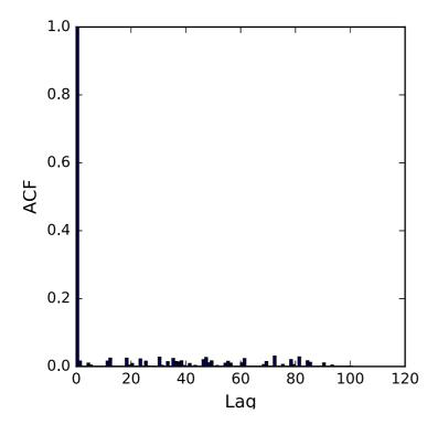
Here the acf value at lag 1 is  $\rho = 0.0154$  and as MCMC algorithms should produce chains resembling an auto-regressive process of order 1 i.e. the value at the current iteration only depends on the last iteration, the value at lag 2 should be approximately  $\rho^2$  (0.000236) and in reality it is -0.0153. Here the chain is only a little correlated.
