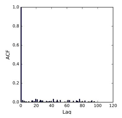
Here the acf value at lag 1 is  $\rho = -0.0051$  and as MCMC algorithms should produce chains resembling an auto-regressive process of order 1 i.e. the value at the current iteration only depends on the last iteration, the value at lag 2 should be approximately  $\rho^2$  (2.6e-05) and in reality it is 0.0208. Here the chain is only a little correlated.
